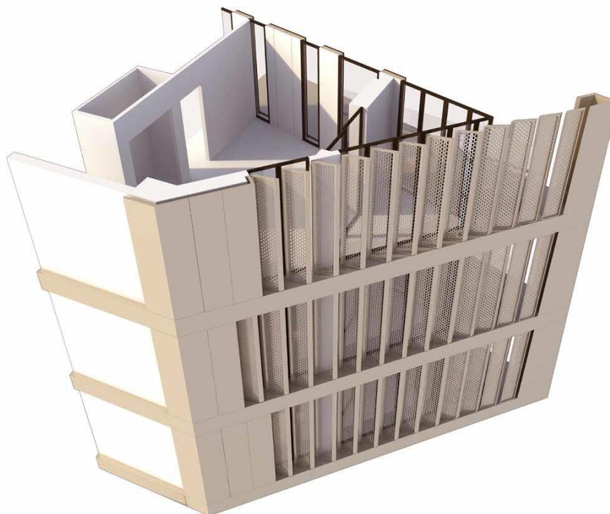
Figure 11. Perforated mesh louvres
